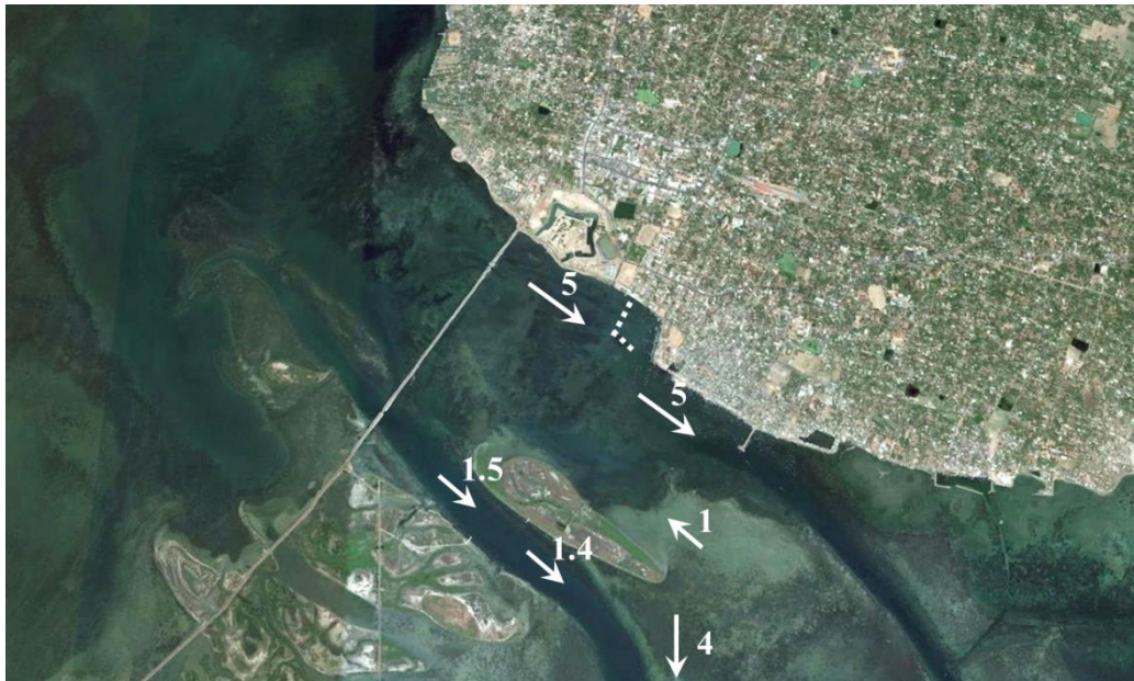
Figure E2. Annual Sediment budget at Gurunagar - white arrows, unit 1000\text{ m}^3/\text{year} . White dashed lines represent the proposed harbour breakwaters (not included in model).
