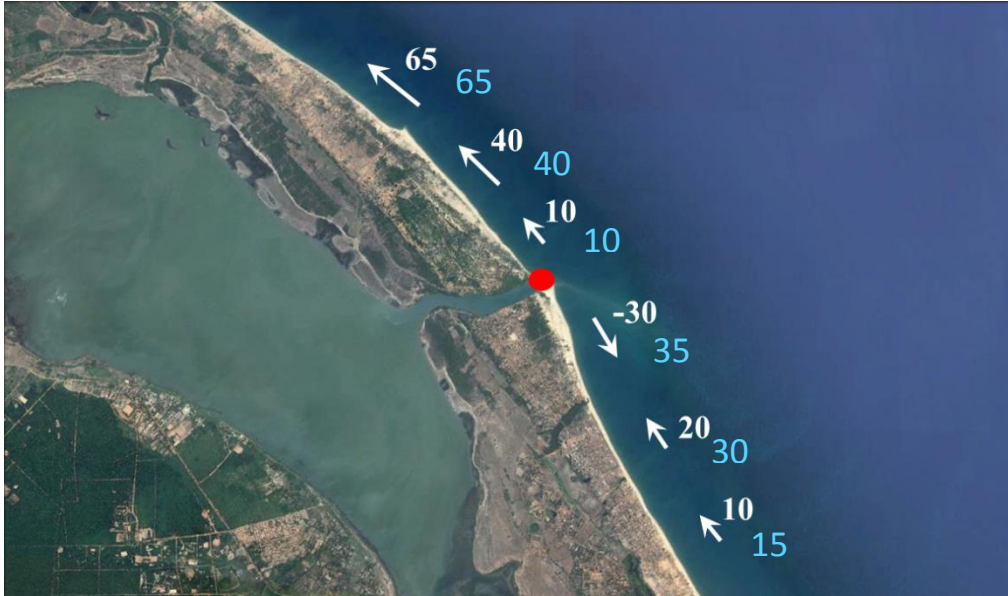
Figure E4. Sediment budget at Mullaitivu – white arrows and numbers show net longshore transport. Gross sediment transport rates are shown in blue numbers, unit – 1000m 3 /year. The red circle shows the earlier proposed harbour location.
