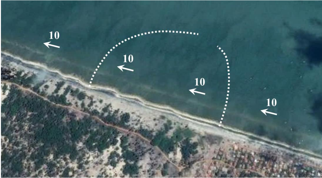
Figure E1. Annual Sediment budget at Pesalai – white arrows, unit – 1000\text{m}^3/\text{year} . White dashed lines represent the proposed harbour breakwaters (not included in the model).
